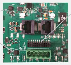
\* VIN pin 20 is not protected and should not be used
