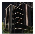
**HB30 Series** Compact form, integral driver enables longer runs, illuminates over 15' Static, RGB, RGBW 4.5-7w/ft. 217-7**00**lm/ft
